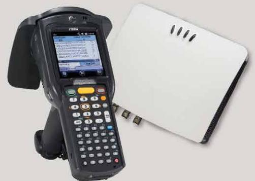
First, RFID avoids the limitations of barcode scanning, which requires line-of-sight access to each barcode and can only be used to scan one item at a time. Instead, RFID tags do not require line-of-site, and multiple RFID tags can be detected and read remotely and simultaneously. They can be read from a variety of distances based on the type of tag and the use of a handheld reader or a fixed RFID reader combined with an antenna.
